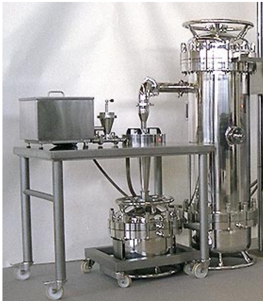
KOMPAK-2, pharma, 10-bar shock resistance
