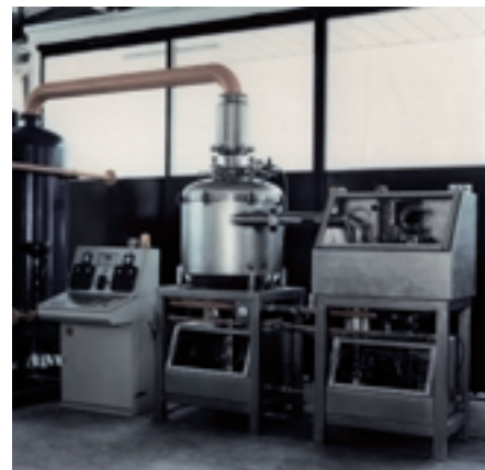
SUPERJET MICRONISER JM3 WITH INERTED, INDEPENDENT GLOVE-BOXES
